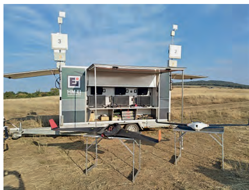
Picture 6: Mobile Flight Control Station and M-8 target UAVs in front on the left; Source: Photo of the HM EI Zrt.
