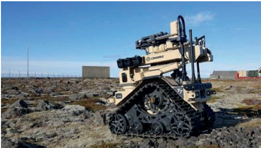
Image 2: L3Harris Technologies T7 explosive ordnance disposal (EOD) robot; Mike Ball: Explosive Ordnance Disposal UGVs Delivered to UK MOD; 06 Jul 2021; https://www.unmannedsystems-technology.com/2021/07/explosive-ordnance-disposal-ugvs-delivered-to-uk-mod/ Downloaded: 18. April 2026
